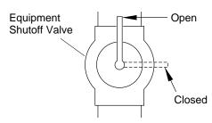
Figure 14 - Equipment Shutoff Valve
